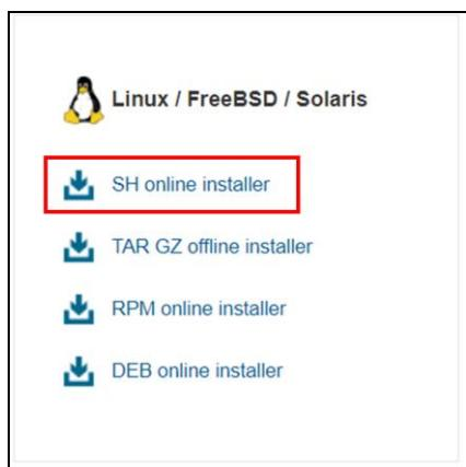
5. Use the **curl** command with the copied link address to download the AhsayOBM installer from the backup service provider's website onto the Linux machine.
