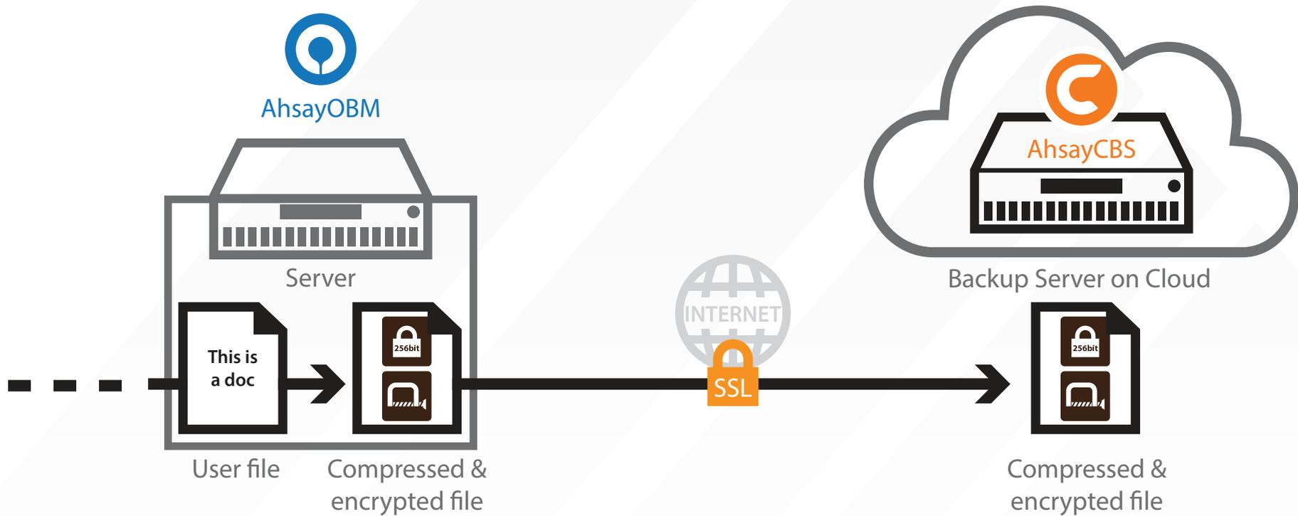
All communications between the AhsayOBM/AhsayACB backup agents and the AhsayCBS server or public cloud storage is via 256 bit SSL (Secure Socket Layer) channel using TLS (Transport Layer Security) v1.2 protocol to ensure that your data is transmitted securely.
